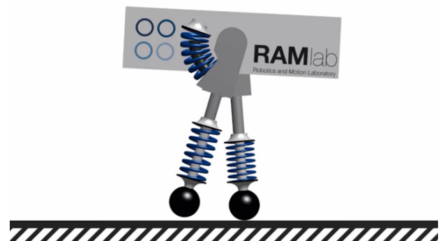
Figure 2: Simplified bipedal model with parallel elastic actuators used in the study.
